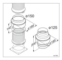
In addition to insulating the exhaust ducting, we recommend that a suitable condensate trap is installed to collect and evaporate any condensate which may occur. Condensate traps are available for Ø 125 mm or Ø 150 mm ducting.
